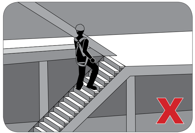
Figure 6.2: Unprotected stairways pose a falling hazard.
