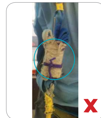
Figure 29: Example of an unsafe practice where an activated energy absorber is being tied up and reused.
