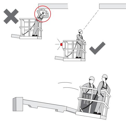
Do not exceed the Safe Working Load and maximum Number of Occupants of the platform specified by the manufacturer.
