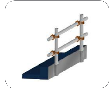
Figure 30: Example of edge protection off the structure.
