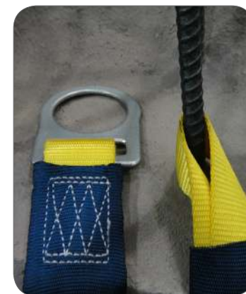
Figure 41: Example of a strap anchor.
